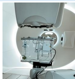
Figure 1. Setup for absorbed dose to water measurement
